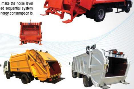
Garbage Compactor cum dump trucks, as the name indicates, are combination of Garbage compactor Trucks & dump Trucks. Unique design of this equipment allows manual loading of garbage as well as Loading through bulk waste lifting machines like Front End Loaders, Excavators, backhoes etc resulting a rapid waste collection & compaction process.
